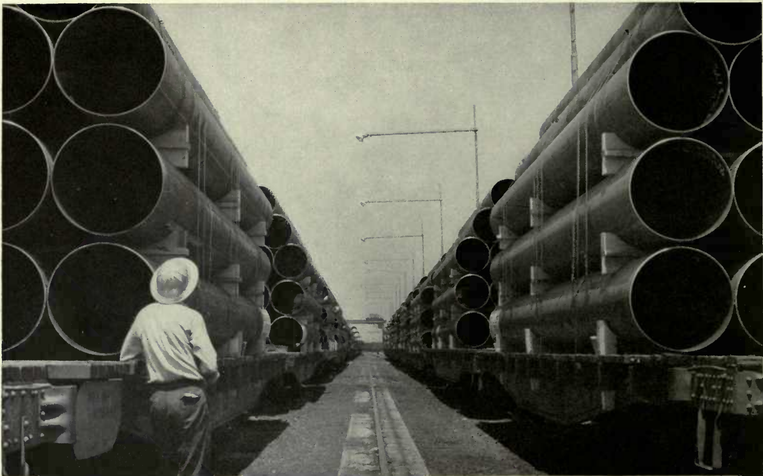
U. S. Steel had the only plant in America capable of making 24-inch seamless steel pipe for the Big Inch pipeline.
